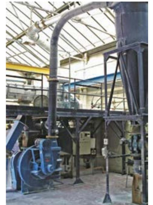
The 8A Dryer-Pulveriser in Atritor's test facility
