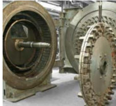
Fitting the rotor in a 20A Dryer-Pulveriser
