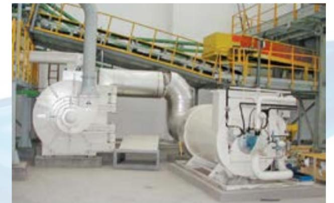
An 18A Dryer-Pulveriser and gas-fired air heater for processing precipitated calcium carbonate (PCC)
