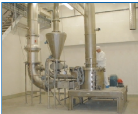
DCM 800 classifier mill is one of a pair processing pharmaceuticals and food ingredients. Special design larger mills are available
