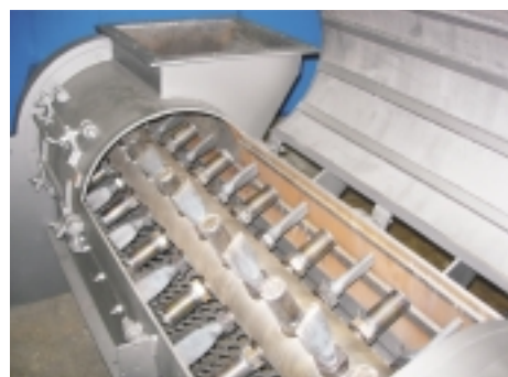
Atritor-Scott Turbo Separator Separates Product from Packaging for Recycling or Disposal.
